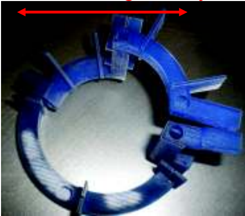
Plastic-wax piece for rapid prototyping
