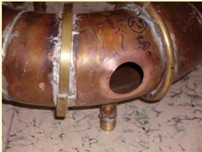
Detail of hole for port and two rings to reinforce the VV
