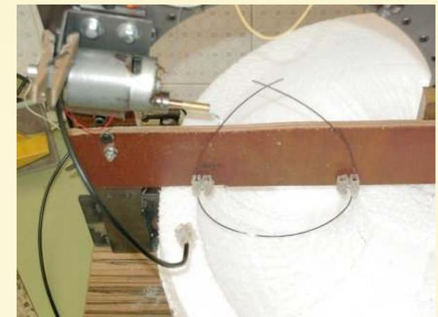
It takes ~2 hours to mechanise a groove 7mm width, 12.5mm depth. Poloidal forward speed adjustable according to slope. Manual (by now) toroidal position
